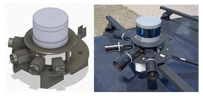
The optics for the cameras are not shown in the Computer Aided Design (CAD). In the current configuration four cameras are facing forward, 20° and 60° angled relative to the forward axis of the car. These four cameras are equipped with a "normal" optic (so it can be approximated using the pinhole model).
