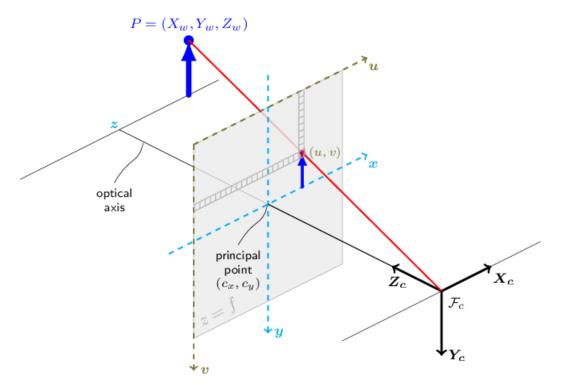
The coordinate system used on the cameras are the OpenCV camera coordinate system. It is originated at the focal point of the camera, and uses a left-handed coordinate system, as shown above. The illustration is taken from the OpenCV documentation, for more information, look at the official OpenCV documentation <u>here</u>. Because of the differences in the systems, a coordinate conversion is needed.
